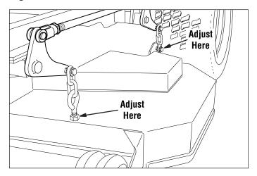
Figure 11. Hanger Chain Adjustment
